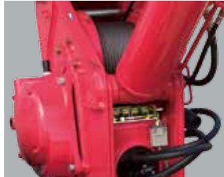
13 Automatic stop for leaving minimum wire rope
