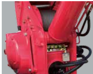
13 Automatic stop for leaving minimum wire rope
